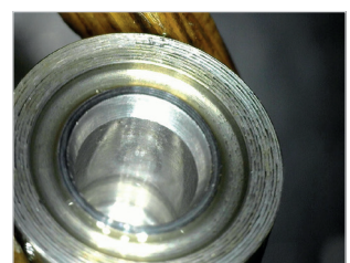
particles on valve seat
