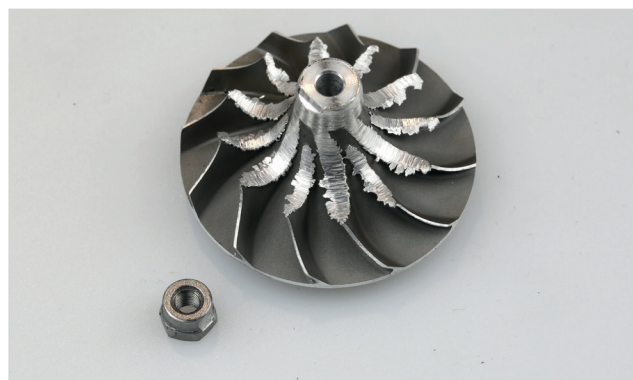
damage to compressor wheel blades
