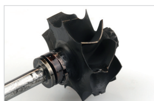
damage to turbine wheel blades
