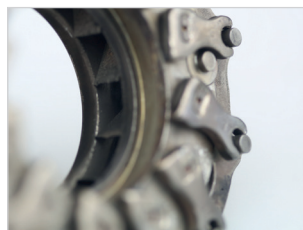
damage to nozzle ring blades
