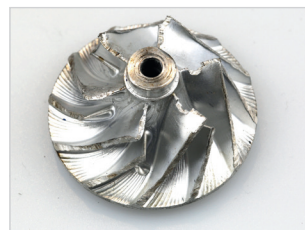
damage to compressor wheel blades
