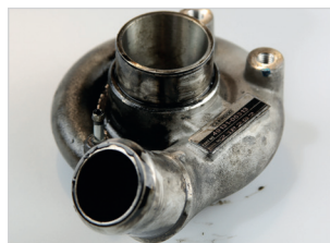
oil in compressor housing
