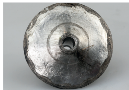
orange peel on back of compressor wheel
